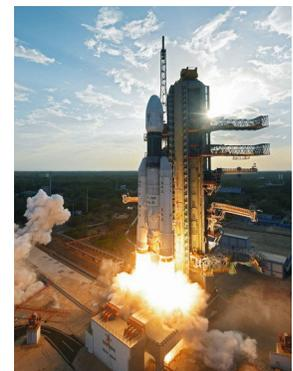
This was the first orbital mission of GSLV Mk III and was mainly intended to evaluate the performance of the vehicle including its fully indigenous cryogenic upper stage during the flight. The cryogenic stage used liquid Hydrogen and liquid Oxygen as propellants with a total loading of 28 tons. The successful launch demonstrates India's ability to launch large payloads and opens up the possibility of increased space exploration and its utilization for the benefit of humanity.
